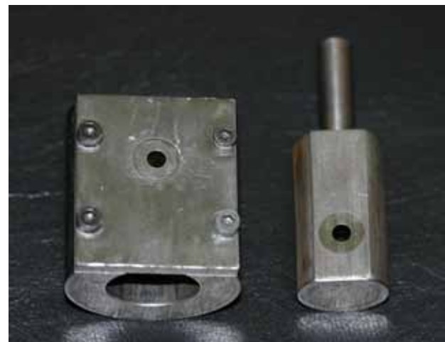
Figure 2a - Device used in the shear bond strength test. (A) internal piece and (B) external piece.
