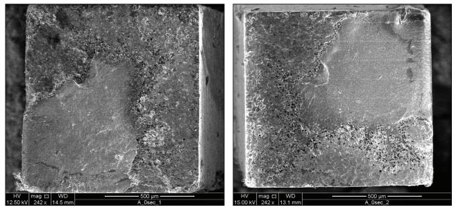
Figure 1- Representative SEM micrograph of the ceramic and composite resin surfaces after the test. The failure mode was classified as cohesive failure of the resin cement, since it is possible to observe resin cement in both half's of the specimen.
