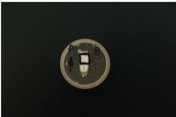
**Figure 1** - Standardized sample: root portion embedded in acrylic resin inside PVC tube. Observe the marked area to be analyzed and the apical-crown direction of the scaling.
