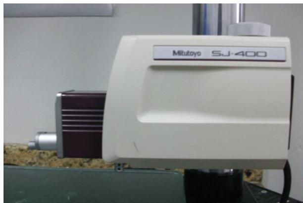
**Figure 2** - Rugosimeter used to measure the roughness degree of the root surfaces.
