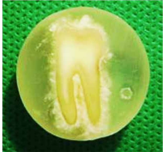
Figure 1 - Specimen preparation. A - Dentin exposed after grinding. B - Resin composite restoration built on dentin.
