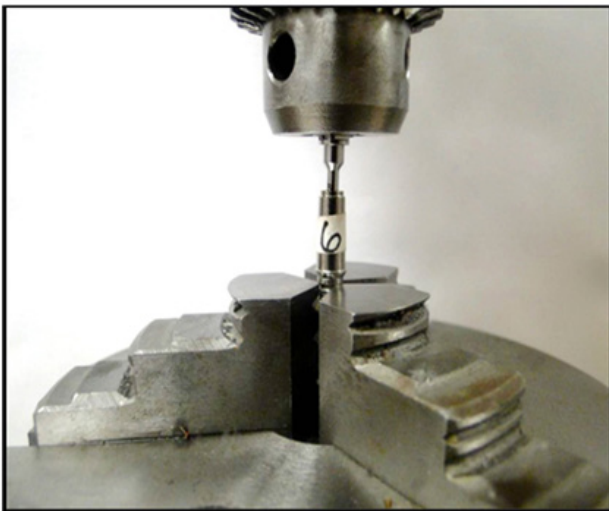
Figure 1 – The specimen was attached to the universal test machine and received torque at a speed of 1 N.cm/s. Techniques referenced in the literature (conventional technique, technique proposed by Breeding et al. [25] and Dixon et al. [2], technique proposed by Sella et al. [18]) were used to perform the torque.
