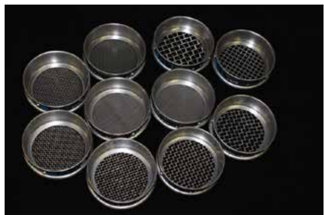
Figure 2 - Ten granulometric sieves in which the particles of Optocal are retained.
