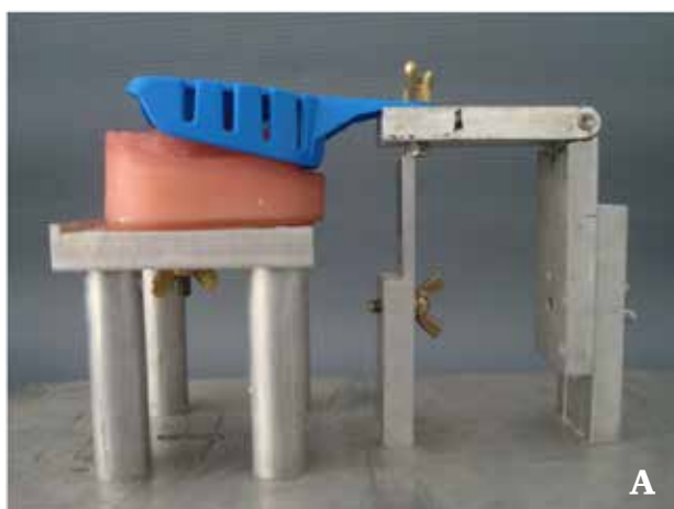
Figure 2 - a) Device used for impression standardization. b) Impression of standard upper model by alginate.
