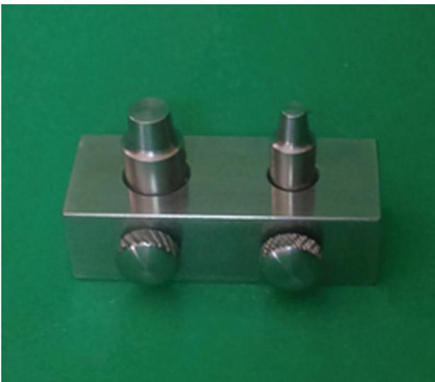
**Figure 1** - The machined stainless steel dies placed in stainless steel holder.
