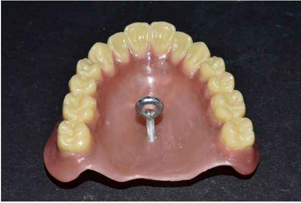
Figure 12 - Inserting the hook for measuring retention in the determined geometric centre.
