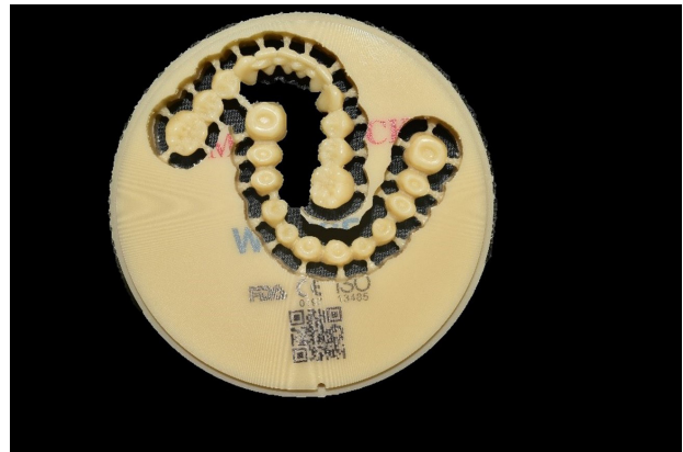
Figure 7 - Milled complete set of artificial teeth.
