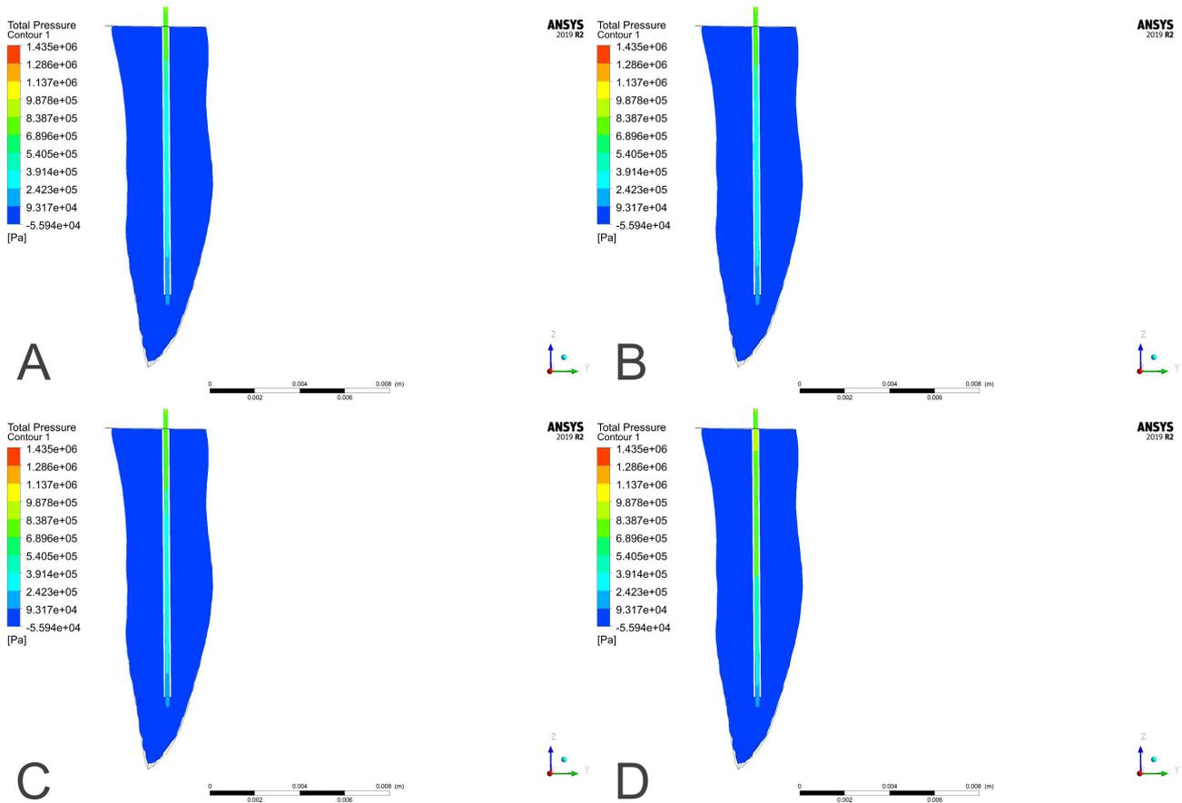
Figure 1 - CFD analysis of apical pressure assessed at different flow rate. A) 1 ml/min, B) 4 ml/min, C) 6 ml/min, D) 12 ml/min.
