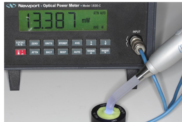
Figure 3 - Photograph of the alignment process of a light polymerizing unit over the zirconia specimen. The process involves the use of a silicone jig over the optical detector, which is connected to a digital optical power meter for the measurement of transmittance.
