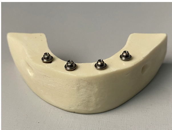
Figure 1 - Polyurethane prototype resembling an edentulous mandible with a flat base and borders with Conexão Torque Hard implants and prosthetic abutments installed.
