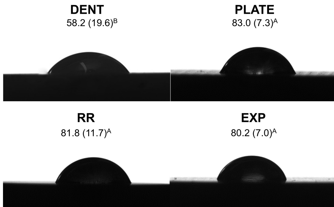
Figure 1. Representative figures, mean and standard deviation of the surfaces contact angle in each group post-etching with phosphoric acid (DENT) and 10% hydrofluoric acid (PLATE, RR and EXP).
