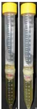
Figure 1 - Specimens A) without and B) with leakage
