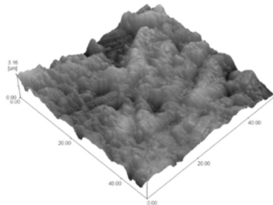
**Figure 6** - Ceramic - Sandblasting at 10 mm.
