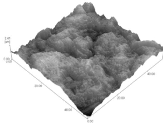
**Figure 5** - Ceramic - Sandblasting at 5 mm.
