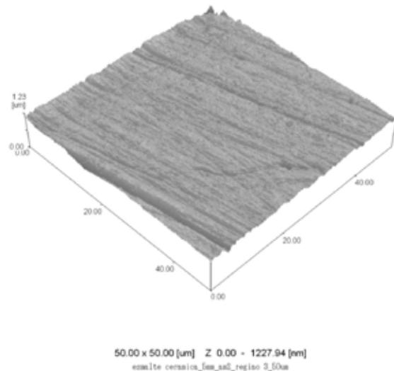
**Figure 1** - Enamel- noSandblasting.
